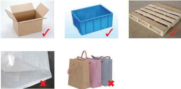
⚠ Objects with a small contact surface i.e. point contact or line contact, may damage the roller (localized abrasion, damage to the tapered sleeve, etc.)
