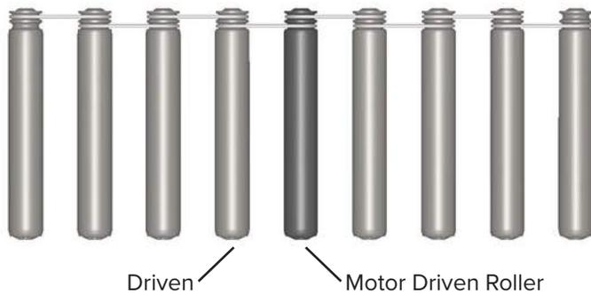
Double Groove Pulley Drive Layout:
